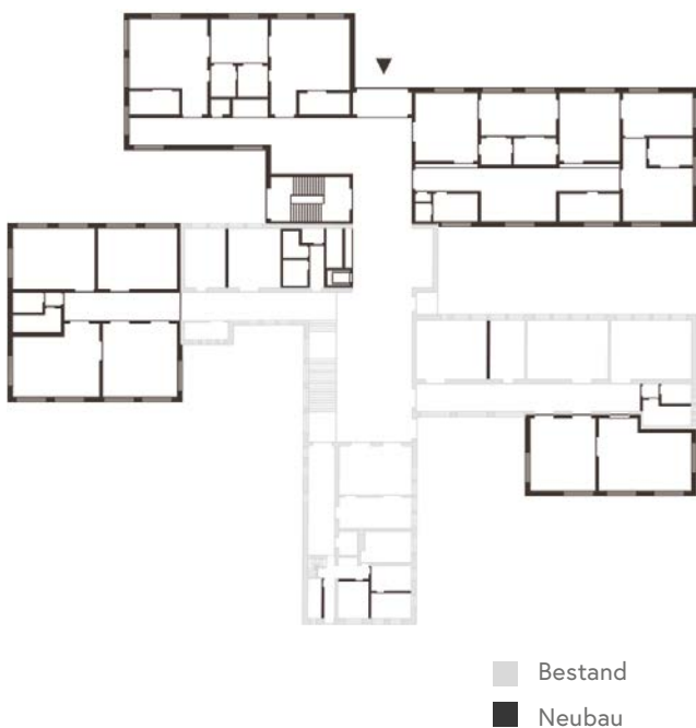
Grundriss Erdgeschoß Quelle: Pedevilla Architects
